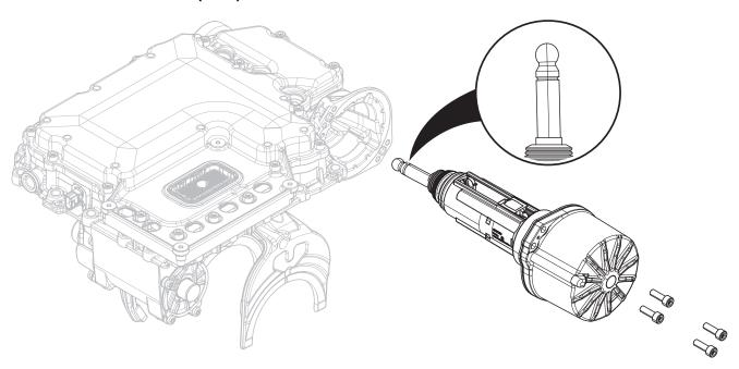
**NOTICE**: Endurant Family LCA's are product specific. The Endurant XD Series LCA push rod is 30mm longer and can be identified by a groove on the end of the LCA push rod. Improperly installing an Endurant HD Series LCA onto an Endurant XD Series Transmission may result in Fault Code 706 FMI 18 setting Active.
