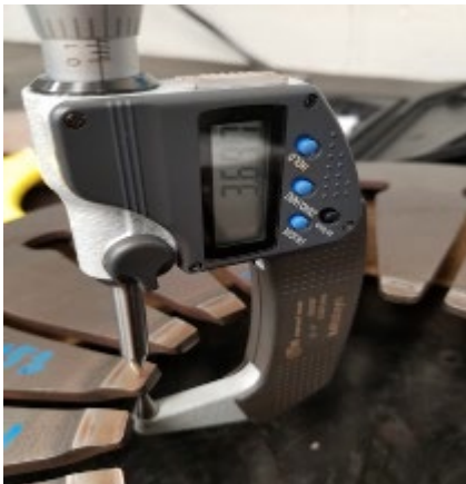
Worn (Less than 4.0mm)
