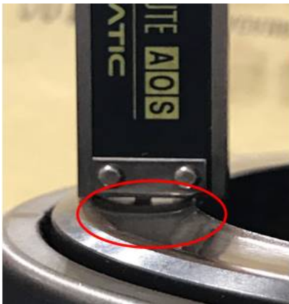
Image C: Release Bearing Face Wear Measurement: “Circumferential” wear
