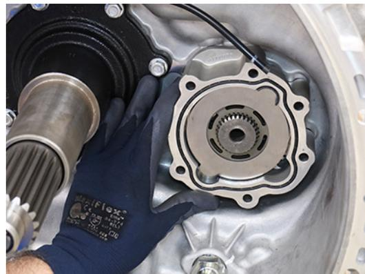
3. If removed, install the Return Spring into the Lower Countershaft.
