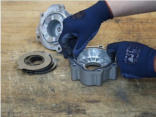
5. Install the inertia brake clutch pack in the order shown below:
