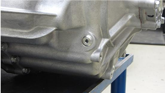
6. Inspect Oil Fill Plug and O-ring for damage. If damaged, replace the Oil Fill Plug; O-ring is serviced with plug.
