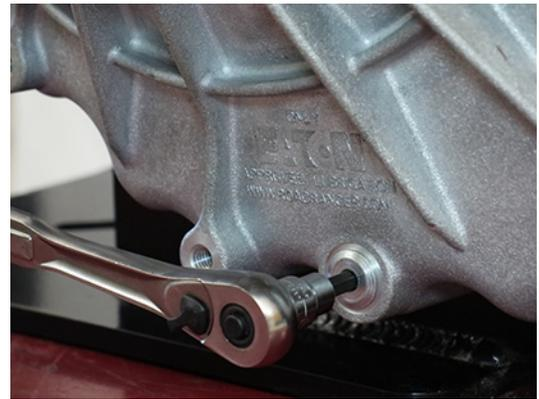
4. Inspect Oil Drain Plug and O-ring for damage. If damaged, replace the Oil Drain Plug; O-ring is serviced with plug.
