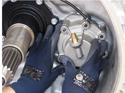
2. While holding the Inertia Brake Housing to the clutch housing, remove the Inertia Brake Cover.
