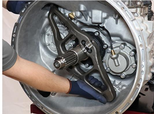
3. Pull to free the upper Clutch Release Yoke socket from the Linear Clutch Actuator (LCA) rod end.
