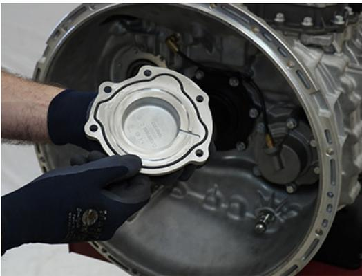
3. Install the new Upper Countershaft Cover and six 13 mm cap screws to the clutch housing and torque to 21-25 Nm (16-19 lb-ft) in a criss-cross pattern.
