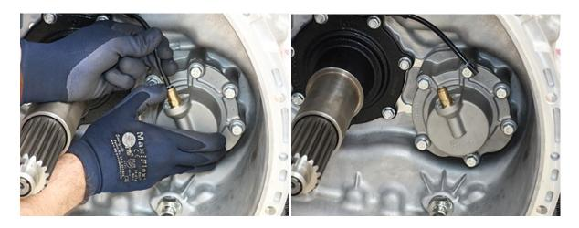
**14.** Inspect Inertia Brake Air Line and fitting for Black and Amber substance.
