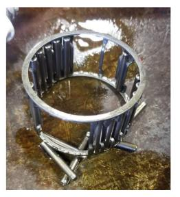
Root Cause: Tool marks on bearing cage bar
