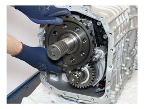
27. Place Upper Shaft Rear Bearing Inner Race onto end of Upper Shaft.
