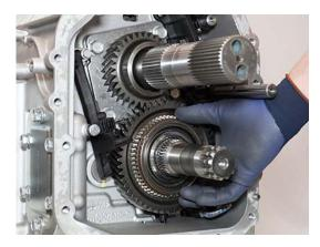
**10.** Assemble Rail C Synchronizer assembly.
