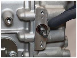
5. Push Rear Housing Cover flush to Main Housing.
