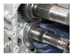
5. Install 6th Gear Bearing on Lower Shaft.
