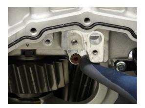
2. Install 2 ACM Alignment Pins (RR1036TR) into Interface Manifold outermost threaded mounting holes.
