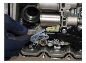
**3.** Remove the 2 Transmission Harness to Main Housing 10 mm cap screws.
