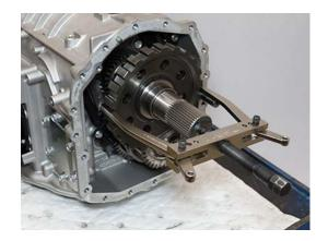
5. Pull off 4th Driven Gear, Park Pawl Gear and Upper Shaft Rear Bearing Inner Race then go to Step 25.
