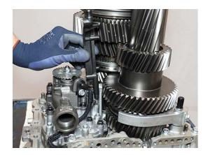
2. Remove 10 Pump 8 mm cap screws.
