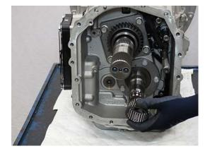
**16.** Rotate Lower Shaft to position 6th Gear Mid-Wall Bearing Spacer and Alignment Ball in 12 o'clock position.
