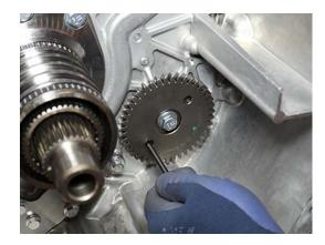
Hold drift securely against Clutch Housing to hold Pump Driven Gear stationary and torque Pump Driven Gear 13 mm cap screw to 32.5-39.5 Nm (24.0-29.1 lb-ft).
