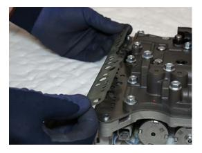
**11.** Inspect ACM to Interface Manifold Gasket for damage. If damaged, replace Gasket.
