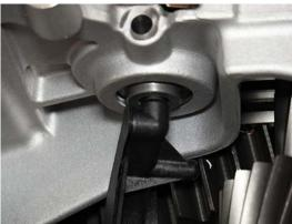
**5.** Align Reverse Idler Shaft to Main Housing to allow installation of the Main Housing to Reverse Idler Shaft cap screw.
