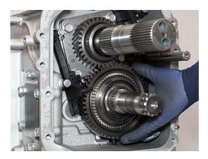
**9.** Install Rail C Synchronizer Blocking Ring onto 6th Gear.
