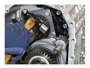
26. Install 4th Driven Gear and Park Pawl Gear assembly on Upper Shaft.
