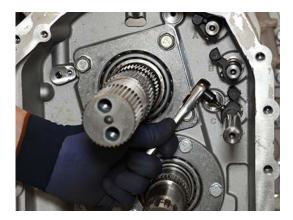
**5.** Remove Shift Rail Magnets A, B and C.
