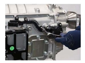
5. Remove TRS assembly from Main Housing and Rear Housing Cover Internal Shift Shaft.
