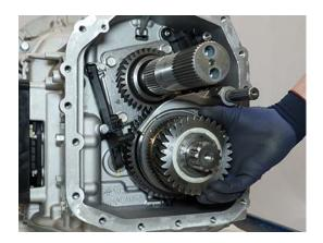
**17.** Place Lower Shaft 4th Gear Inner Sleeve Driver (RR1040TR) on Lower Shaft and against 4th Gear Captured Inner Race.
