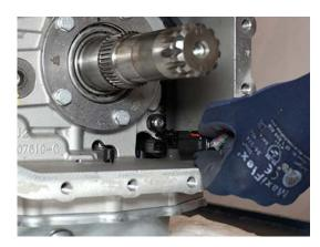
2. Remove 4, 3-Rail Position Sensor T30 torx head screws.
