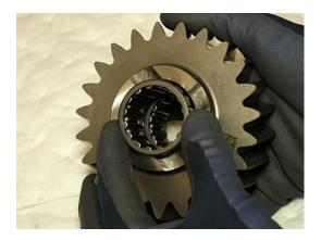
**3.** Install Reverse Idler Gear assembly into Main Housing.
