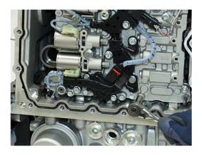
**10.** Install ACM Retainer Tab, O-ring isolator, and 13 mm cap screw and hand tighten.
