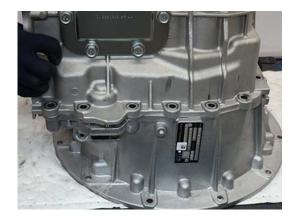
6. Install 16 external and 5 internal Main Housing 16 mm cap screws and torque to 44.5-51.5 Nm (32.8-38 lb-ft) in a crisscross pattern.
