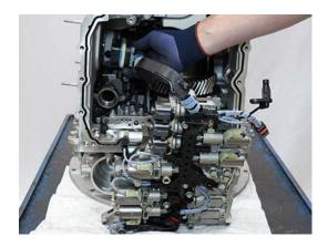
**5.** Route 74-Way Transmission Harness Connector into 74-Way Connector Retainer.
