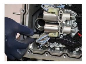
**18.** Connect 8-Way Transmission Harness Connector to 90-degree pass-through connector and latch red lock tab.
