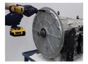
2. Locate 2 jackscrew threaded holes in Front Cover at the 2 & 8 o'clock positions.
