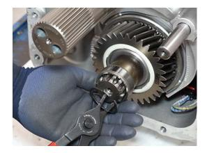
**12.** Install puller large jaws into puller crossarm as shown.
