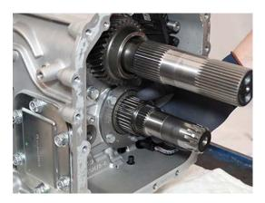
6. Install Rear Lube Bar into Main Housing and Reverse Idler Shaft.
