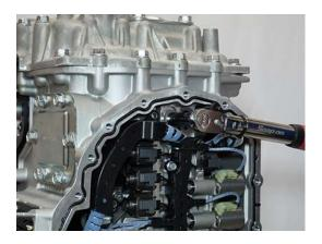
**15.** Install Output Speed Sensor and 10 mm cap screw into Main Housing and torque screw to 8.8-10.4 Nm (77.9-92 lb-in).
