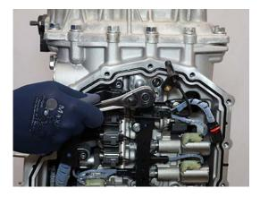
6. Remove ACM Retainer Tab and O-ring isolator.
