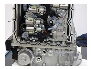
**13.** Torque all 6 ACM to Interface Manifold 10 mm cap screws to 8.8-10.4 Nm (77.9-92 lb-in).
