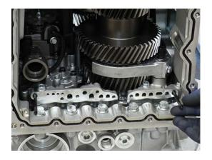
**3.** Orient and install ACM to Interface Manifold Gasket on ACM Dowel Pins.
