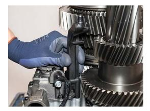
5. Clean Rail D Position Sensor Magnet (in place) of any metal shavings or debris.
