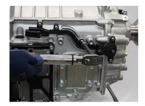
**3.** Install Transmission Cable Shift Lever on Internal Shift Shaft.
