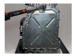
8. Ensure Oil Drain Plug is installed. If not, Install the Oil Drain Plug and torque to 27.5-32.5 Nm (20.3-24 lb-ft)
