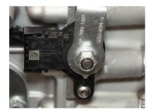
2. Use hand tools to remove Transmission Cable Shift Lever retaining nut.
