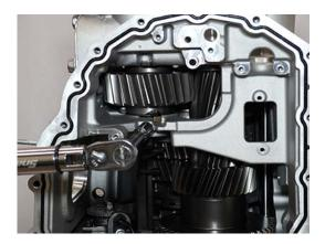
7. Remove the M12x1.75x60 bolt used during disassembly/assembly from Reverse Idler Shaft.
