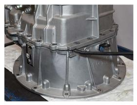
**3.** Lift and remove Main Housing from Clutch Housing.
