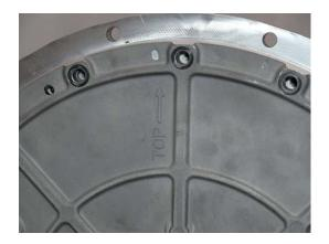
7. Push Front Cover flush to Clutch Housing.
