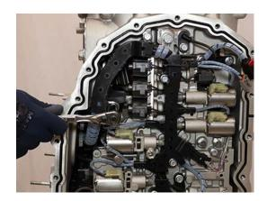
4. Remove Output Speed Sensor 10 mm cap screw and pull Output Speed Sensor free from Main Housing.
