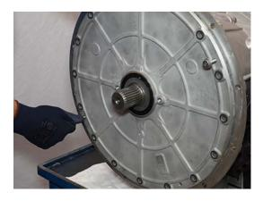
**4.** Hand tighten jackscrews equally in an alternating pattern until Front Cover separates from Clutch Housing, then remove jackscrews.
