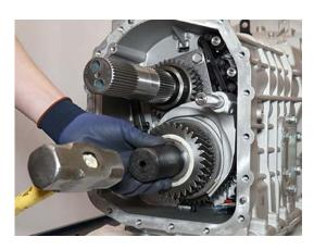
**19.** Install Spacer onto Lower Shaft.
