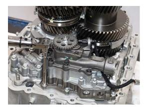
4. Install Main Housing Spray Bar into Pump outlet aligning molded-in cap over Pump cap screw head.
