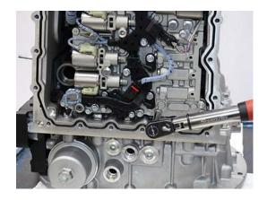
**14.** Torque ACM Retainer Tab 13 mm cap screw to 20.5-25.5 Nm (15.14-18 lb-ft).
