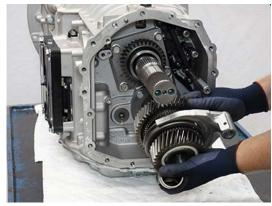
**15.** Remove 6th Gear Bearing from Lower Shaft.
