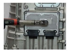
**3.** Install TCM Cover with 4 nuts over TCM studs and torque to 8.8-10.4 Nm (77.9-92 lb-in) in a crisscross pattern.
