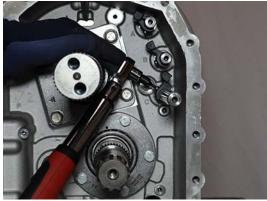
**3.** Position 3-Rail Position Sensor on Main Housing Mid-Wall.
