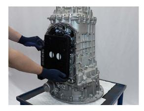
**5.** Install Sump Pan Seal into Main Housing recess if previously removed.
