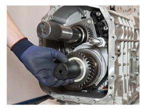
**18.** Drive 4th Gear assembly onto Lower Shaft.
