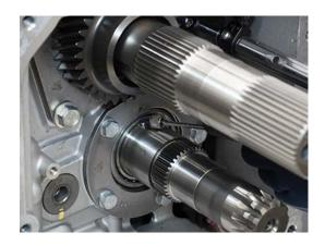
**19.** Remove 6th Driven Gear from Upper Shaft.
