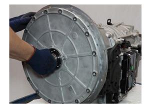
5. Rotate and push DCM Input Shaft to align DCM onto both transmission Input Shafts and the Pump Driven Gear.
