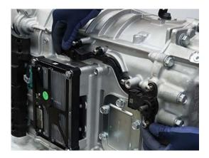
2. Install 5 TRS Harness Bracket to T30 torx head screws and torque to 8.8-10.4 Nm (77.9-92 lb-in).
