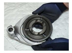
**12.** Install Rail C Synchronizer assembly with Rail C Shift Yoke on Lower Shaft and Shift Rail C.
