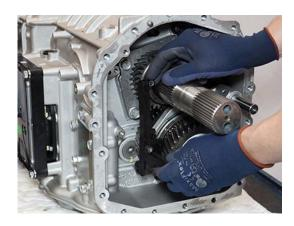
8. Install Shift Rail Actuation Tool (RR1039TR) into Shift Rail C.
