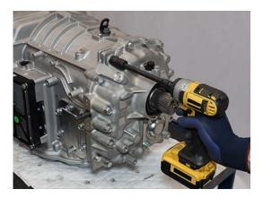
**3.** Separate Rear Housing Cover from Main Housing at 2 pry points.
