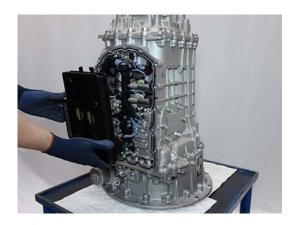
4. Inspect Sump Pan Seal (in place) for damage. If damaged, replace seal.
