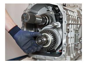
21. Use Lower Shaft Rear Bearing Inner Race Driver (RR1040TR) to drive Lower Shaft Rear Bearing Inner Race onto Lower Shaft.
