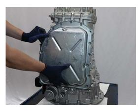
7. Install 20 Sump Pan13 mm cap screws and torque to 27.5-31.5 Nm (20.2-23.2 lb-ft) in a crisscross pattern.
