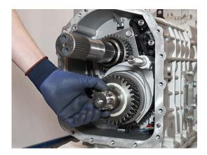
**20.** Place Lower Shaft Rear Bearing Inner Race onto end of Lower Shaft.
