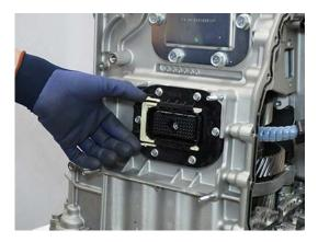
7. Position ACM onto ACM Alignment Pins (RR1036TR).
