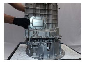
**5.** Push Main Housing flush to Clutch Housing.
