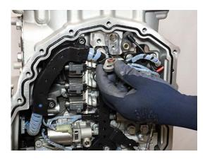
7. Remove 6 ACM to Interface Manifold 10 mm cap screws.
