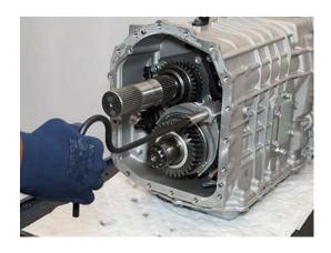
24. Place Rail C Synchronizer Sleeve, Rail C Shift Yoke and Shift Rail C into the 4th Gear position then remove Shift Rail Actuation Tool (RR1039TR).
