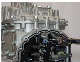
**16.** Install 2 Transmission Harness to Main Housing 10 mm cap screws and torque to 8.8-10.4 Nm (77.9-92 lb-in).
