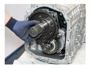
28. Use Upper Shaft Rear Bearing Inner Race Driver (RR1041TR) to drive Upper Shaft Rear Bearing Inner Race onto Upper Shaft.
