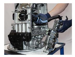
9. Remove ACM rear lubrication O-ring.Note: If O-ring is missing it may be located on ACM.
