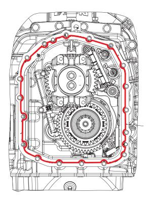
4. Install Rear Housing Cover onto Upper Shaft, Lower Shaft and Main Housing Dowel Pins.
