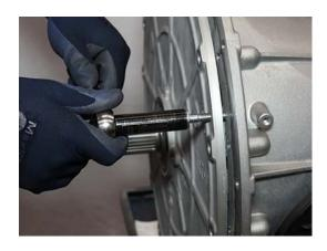
**5.** Carefully pull and remove Front Cover/DCM assembly from Clutch Housing.
