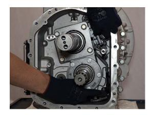
4. Install 4, 3-Rail Position Sensor T30 torx head screws and torque to 8.8-10.4 Nm (77.9-92 lb-in).
