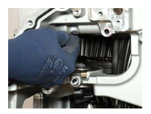
2. Install Reverse Idler Gear Bearings into Reverse Idler Gear.
