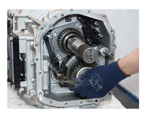
7. Remove Rear Lube Bar from Main Housing and Reverse Idler Shaft.
