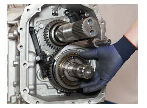
**15.** Install 4th Gear Bearing and Captured Inner Race into 4th Gear.
