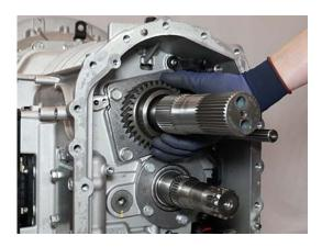
2. Rotate Lower Shaft until 6th Gear Mid-Wall Bearing Spacer Alignment Ball locating hole is in 12 o'clock position.
