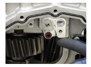
**10.** Remove ACM to Interface Manifold Gasket.
