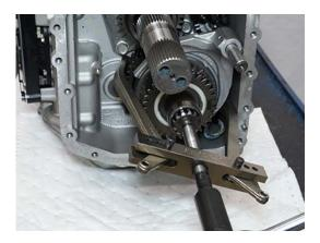
**14.** Pull off 6th Gear, Rail C Synchronizer assembly, 4th Gear, Rail C Shift Yoke and Lower Shaft Rear Bearing Inner Race.
