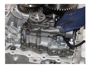
**3.** Install 10 Pump 8 mm cap screws and torque to 8.8-10.4 Nm (77.9-92 lb-in) in a crisscross pattern.
