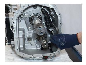
**4.** Remove the 3 Shift Rail Magnet T20 torx head screws from Shift Rails A, B and C.
