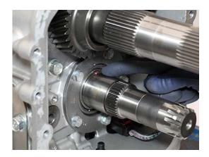
4. Install 6th Gear Mid-Wall Bearing Spacer on Lower Shaft.
