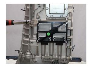
**2.** Unscrew the 7 mm jackscrew and remove TCM from transmission.
