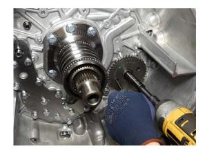
4. Remove Pump Driven Gear.
