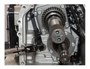
8. Install 6th Gear on Lower Shaft.
