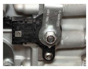
3. Remove Transmission Cable Shift Lever.
