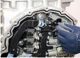
5. Remove the ACM Retainer Tab 13 mm cap screw.
