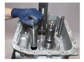
**3.** Remove Reverse Idler Gear, Bearings, and Thrust Washers.
