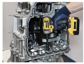
**2.** Separate Main Housing from Clutch Housing at 3 pry points.
