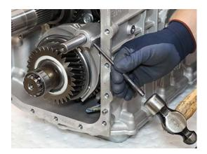
**11.** Remove Lower Shaft Rear Bearing Inner Race Snap Ring from Lower Shaft and discard.
