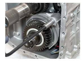
**9.** Pull Shift Rail C to engage Rail C Synchronizer Sleeve onto 4th Gear, remove Shift Rail Actuation Tool (RR1039TR).
