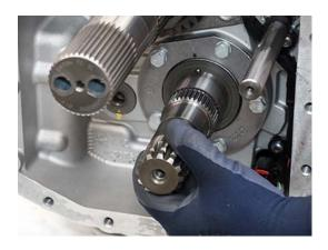
**17.** Remove 6th Gear Mid-Wall Bearing Spacer.
