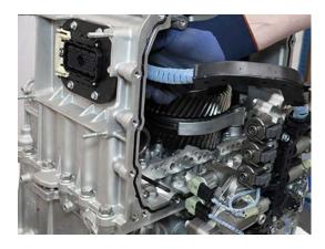
**6.** Latch 74-Way Connector Retainer to 74-Way Transmission Harness Connector.
