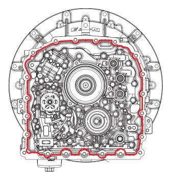
**4.** Lower Main Housing onto Upper Shaft, Lower Shaft, and Clutch Housing Dowel Pins.
