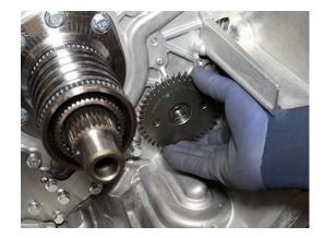
2. Install Pump Driven Gear 13 mm cap screw and hand tighten.
