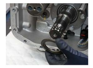
**18.** Use a magnet to remove 6th Gear Mid-Wall Spacer Alignment Ball.
