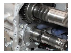
**3.** Install Mid-Wall Bearing Spacer Alignment Ball on Lower Shaft.
