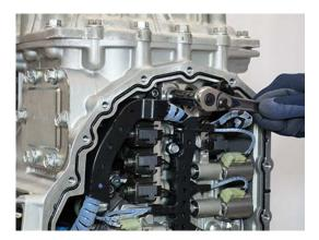
**11.** Remove the 2 ACM Alignment Pins (RR1036TR) from Interface Manifold outermost threaded mounting holes.
