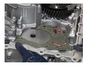
**2.** Align Pump with small Clutch Housing Dowel Pins and install Pump.
