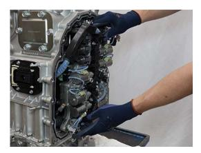
**8.** Push ACM flush to Interface Manifold and Main Housing rear lubrication O-ring.
