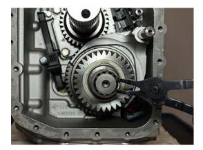
23. Install Shift Rail Actuation Tool (RR1039TR) into Shift Rail C.
