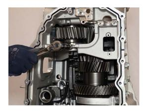
2. Install an M12x1.75x60 bolt into Reverse Idler Shaft and lift to remove Reverse Idler Shaft from Main Housing.
