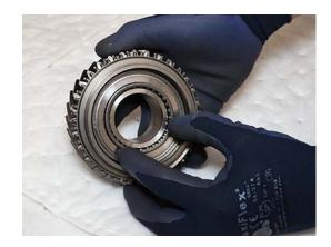
**16.** Place 4th Gear assembly onto Lower Shaft.
