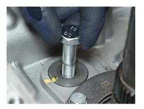
6. Install Reverse Idler Shaft 13 mm cap screw and torque to 27.5-31.5 Nm (20.2-23.2 lb-ft).
