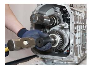
22. Install new Ring on Lower Shaft.
