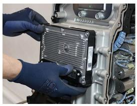
**3.** Unlatch 74-Way Connector Retainer from 74-Way Transmission Harness Connector.
