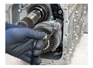
**10.** Drive out Rail C Shift Yoke Roll Pin with 7/32 in. (5.5 mm) roll pin punch.
