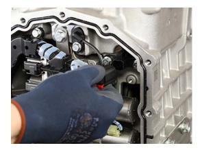
2. Disconnect 2-Way Transmission Harness Connector from Engine Speed Sensor Connector.
