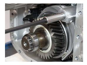
**25.** Install Rail C Shift Yoke Roll Pin.
