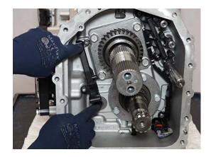
7. Install 2 Rear Lube Bar 10 mm cap screws and torque to 8.8-10.4 Nm (77.9-92 lb-in).
