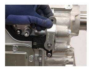
4. Use hand tools to install the Transmission Cable Shift Lever retaining nut on Internal Shift Shaft and torque nut to 20.5-25.5 Nm (15.1-18.8 lb-ft).
