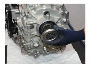
2. Remove 18 Rear Housing Cover 16mm cap screws.
