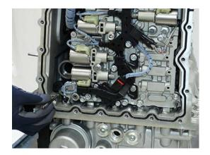
**12.** Install the 2 remaining ACM to Interface Manifold 10 mm cap screws into Interface Manifold outermost threaded mounting holes and hand tighten.
