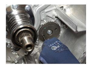
2. Hold drift securely against Clutch Housing to hold Pump Driven Gear stationary.
