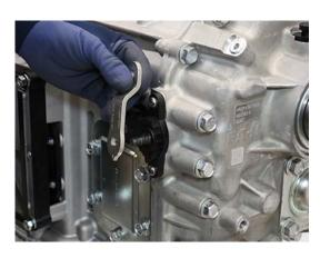
4. Remove 5 TRS Harness Bracket T30 torx head screws.
