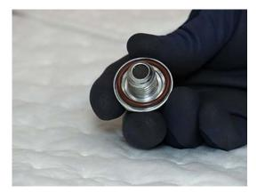
6. Install the Oil Drain Plug and torque to 27.5-32.5 Nm (20.3-24 lb-ft)
