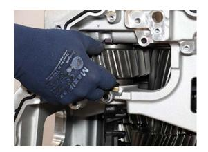
4. Install Reverse Idler Shaft into Main Housing and onto Main Housing Spray Bar.
