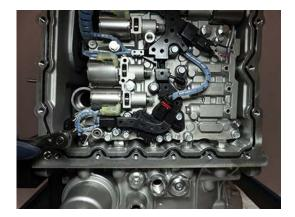
8. Remove ACM/Transmission Harness assembly from Main Housing.
