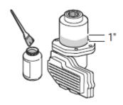
4. Install ECA into the clutch housing bore. Position the ECA so the alignment tab will engage the slot in the clutch housing. Push the ECA straight up far enough that the alignment tab will clear the clutch housing and the ECA can be rotated to align the holes for the cap screws.
