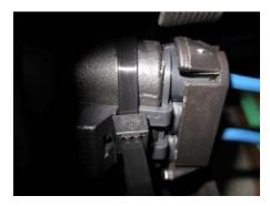
Important: Ensure that the cable tie locking mechanism is positioned directly over the locking tab of each connector.
