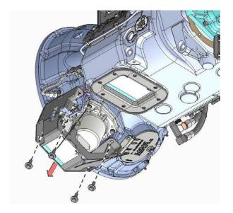
4. Disconnect 3-way vehicle harness connector and 8-way transmission harness
