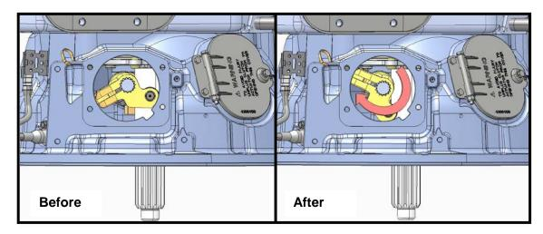
**3.** Apply a 1" band of anti-seize to the barrel of the ECA.
