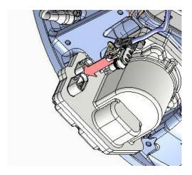
7. Install a cable tie to both 3-way and 8-way connectors.
