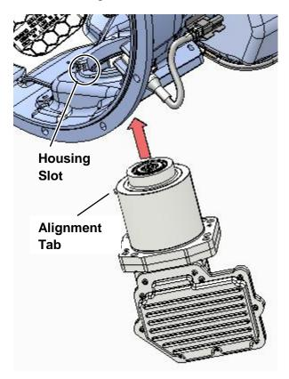
5. Align all four cap screw holes and install cap screws to secure the ECA to the transmission clutch housing and tighten to 35-45 lb-ft (47-61 Nm).
