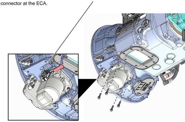
**5.** Remove all 4 cap screws that secure the ECA to the transmission clutch housing.
