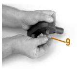
10. Install drive gear on drive shaft, aligning keyway on drive gear with key on drive shaft.
