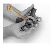
13. Install integral oil pump retainer over alignment pin inside of case, bore retainer facing rear of case.
