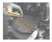
4. Tighten the capscrews to 7 lbs. in. of torque.
