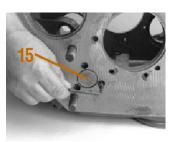
16. Replace o-ring on suction tube and install tube under case rib and into integral oil pump. Bend tube lock on suction tube over case rib.
