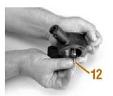
13. Remove the drive shaft from integral oil pump housing. If necessary, remove rear drive gear retention snap ring from drive shaft.
