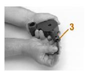
4. Secure oil pump housing in a vice. Depress spring in housing bore and relief valve retention roll pin into roll pin bore.
