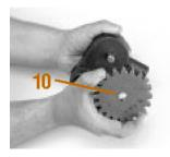
11. Install outer drive gear retention snap ring in the drive shaft groove.
