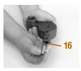
If necessary, front case plug can be removed from case by driving the plug through the front of case. Remove o-ring from outside diameter of plug if necessary.
